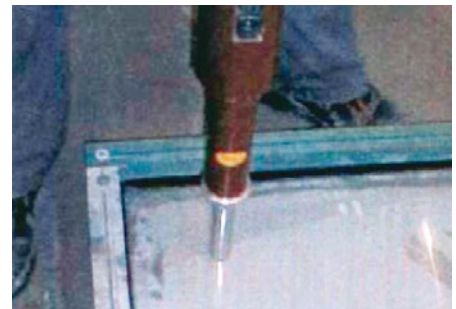
POINT 1 - EDGE IMPACT WITH CONCRETE TESTING HAMMER
