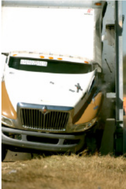
DAMAGED AREAS SHOW HOW THE DURISOL®-ALUMINUM MASH TL-4 SYSTEM REDUCES THE SEVERITY OF THE CRASH
