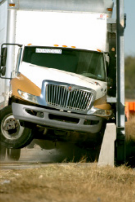
THE DURISOL®-ALUMINUM MASH TL-4 SYSTEM STABILIZES THE VEHICLE AFTER IMPACT
