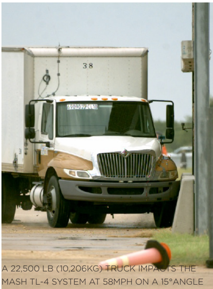
THE DURISOL® MASH TL-4 SYSTEM STABILIZES THE VEHICLE AFTER IMPACT
