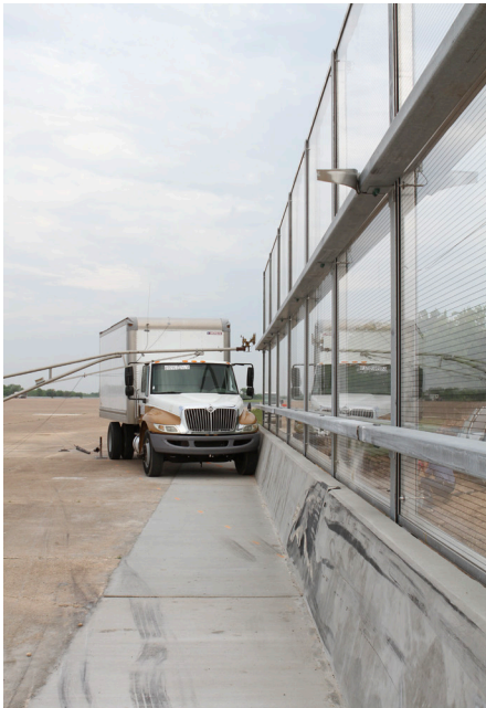
A 22,180LBS (10,060KG) TRUCK IMPACTS THE MASH TL-4 SYSTEM AT 58MPH ON A 15° ANGLE
